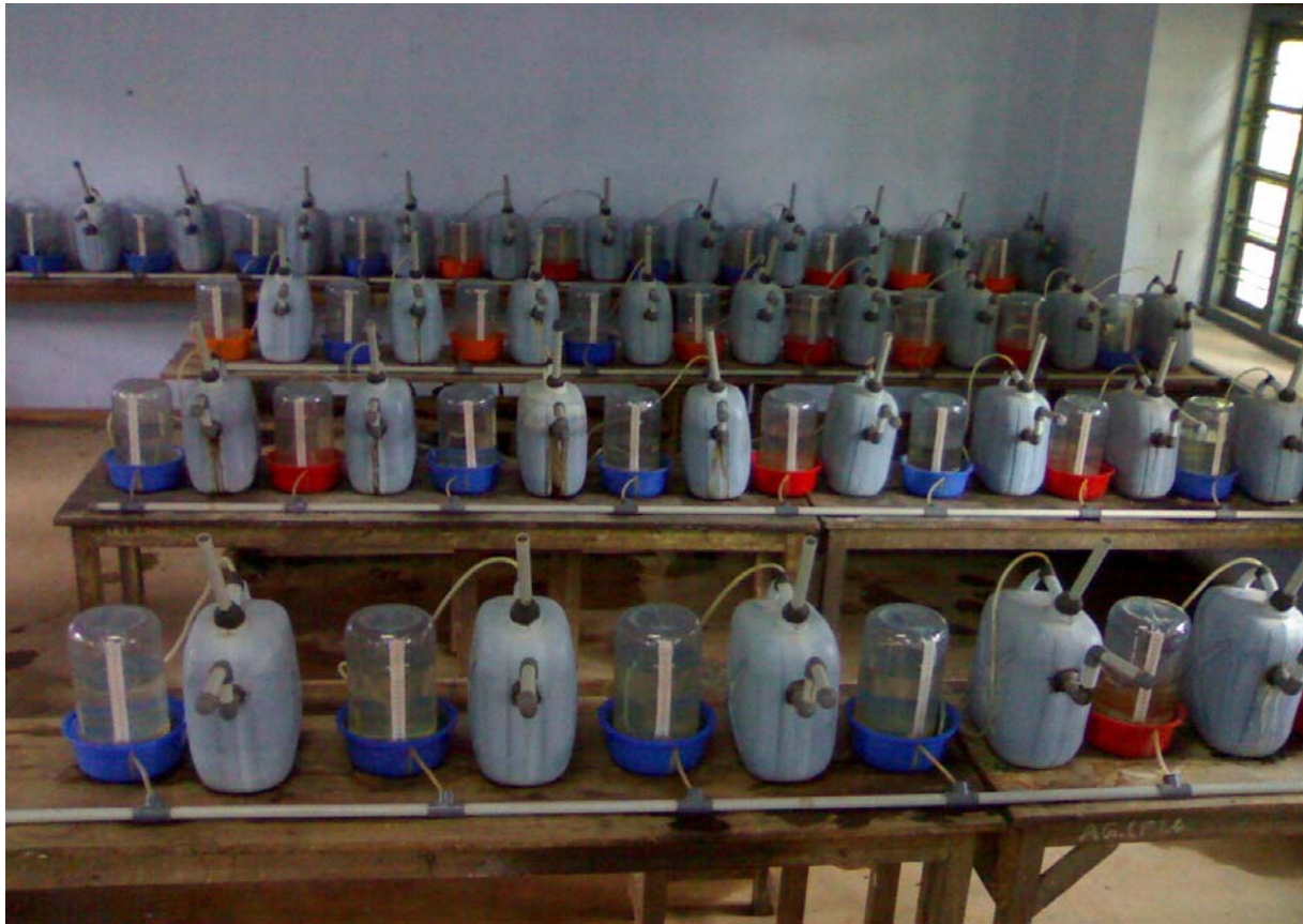
Plate 3.6 Arrangement of digesters for media selection study
