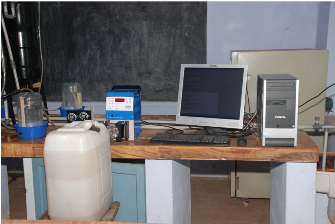
Plate 3.11 Computer controlled feeding system for the bioreactors
