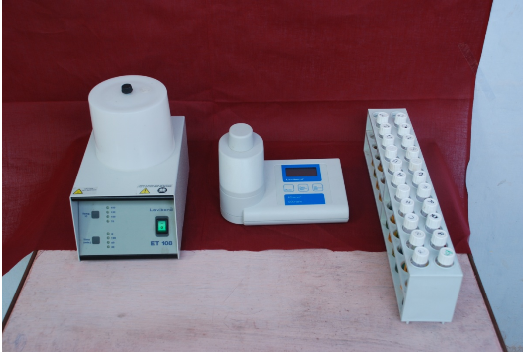
Plate 3.1 Lovibond COD-reactor ET108
