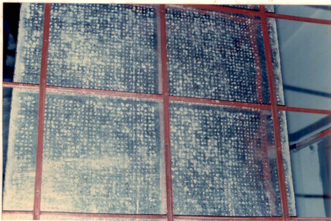
Plate 2. Close view of the wire loops in the drop forming tank
