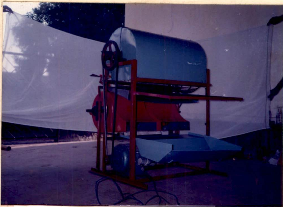
Plate No.6 A view of the developed low cost thresher cum winnower
