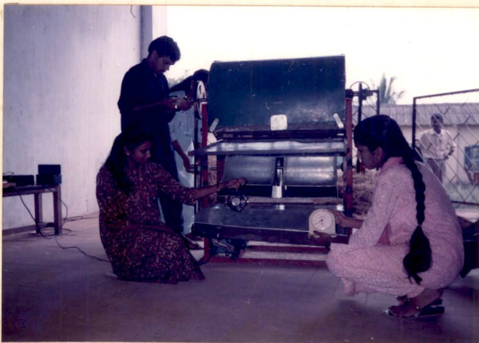
Plate No.9 Testing of the thresher cum winnower under no load condition
