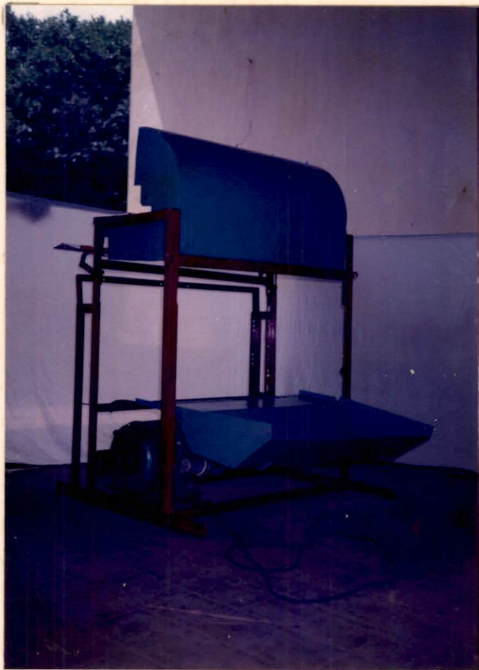
Plate No.5 Main frame and collecting tray
