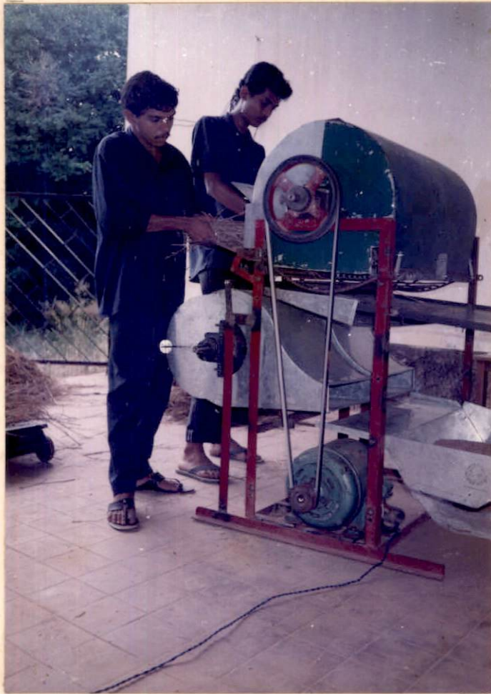
Plate No.10 Field evaluation of the thresher cum winnower under load conditions
