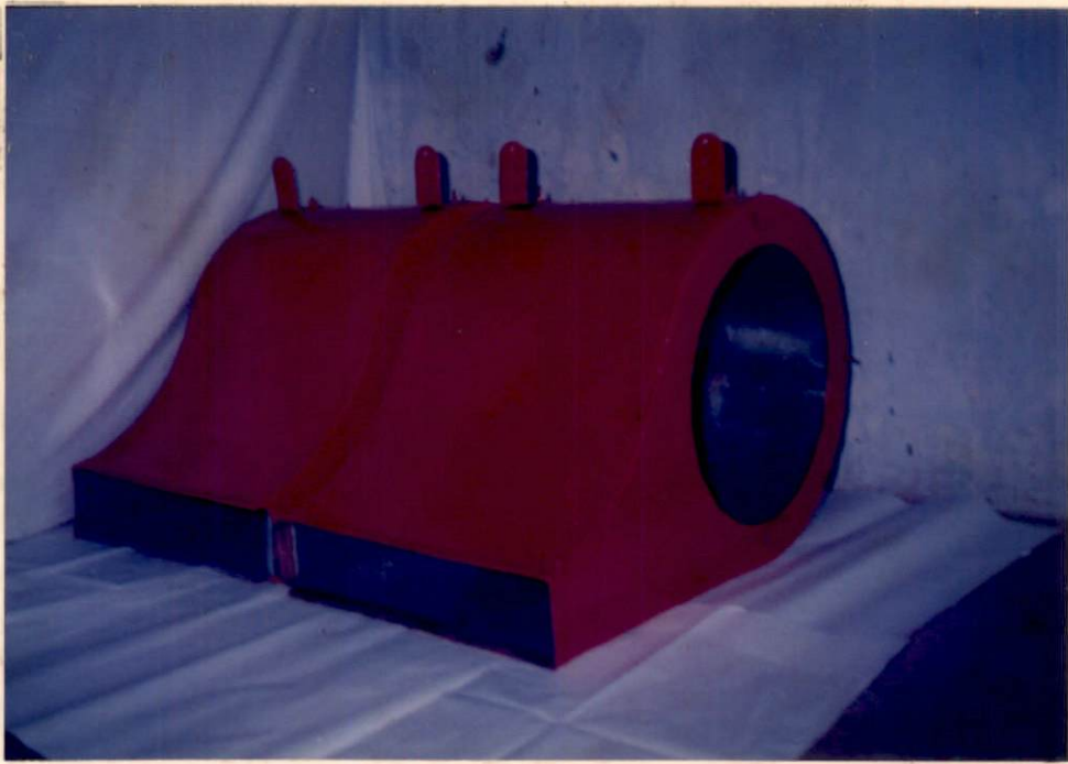
Plate No.3 Spiral casing of the blower
