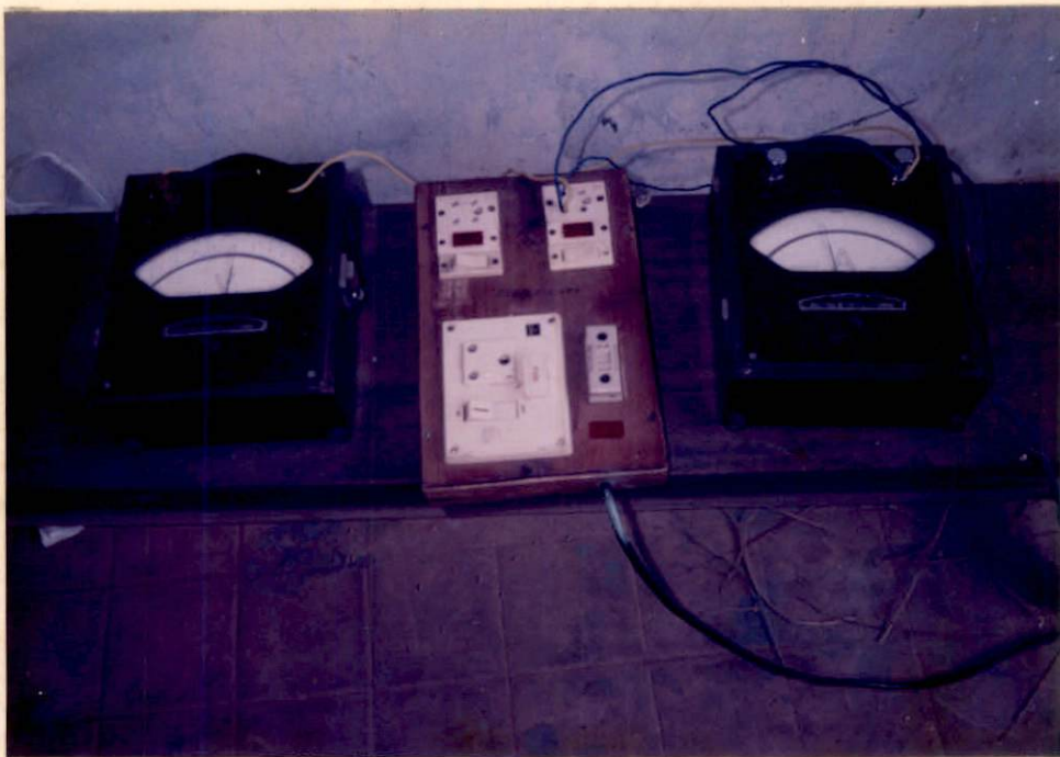
Plate No.8 Set-up for measurement of power requirement of the thresher
