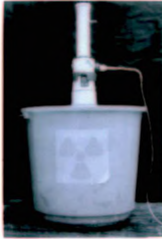
Plate 7 Field dispenser for ^{32}\text{P} application
