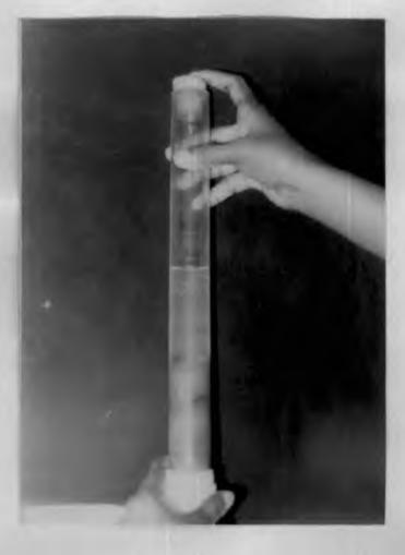
Fig. 2. PVC core tube used for collection of meiobenthos samples.
