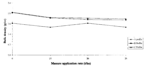
Fig.59 Bulk density values of sandy loam at different profile levels soil under 60 mm/h rainfall intensity.
