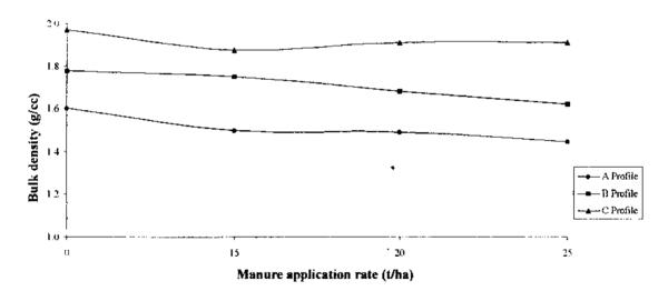
Fig. 60 Bulk density values of clay loam soil at different profile levels under 30 mm/h rainfall intensity.
