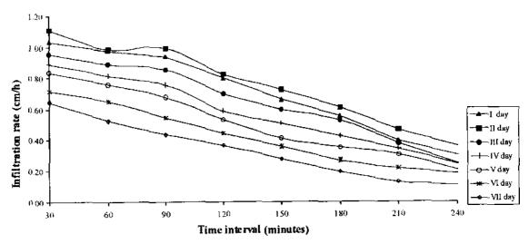
Fig. 9 Infiltration rates of sandy loam soil at 45 mm/h rainfall intensity with 15 t/ha manure application rate.
