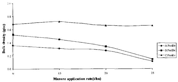
Fig. 57 Bulk density values at different profile levels for sandy loam soil at 30 mm/h rainfall intensity.
