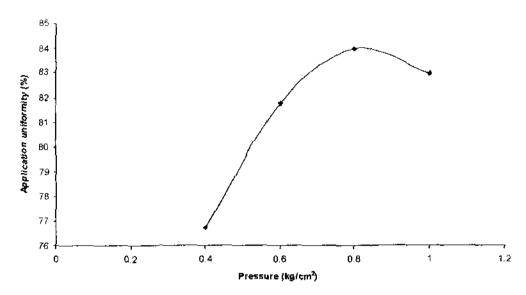
Fig.1 Calibration curve for application uniformity of the rainfall simulator
