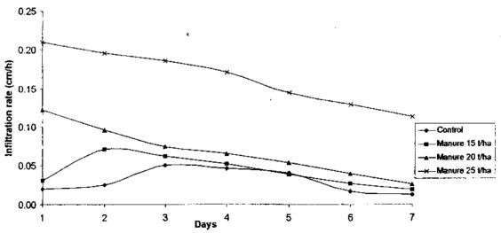
Fig.32 Average daily infiltration rate of clay loam soil at 60 mm/h rainfall intensity.
