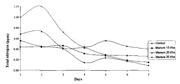
Fig.55 Total nitrogen content of the runoff water of clay loam soil at 45 mm/h rainfall intensity.
