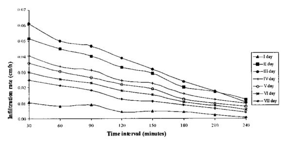
Fig. 23 Infiltration rates of clay loam soil at 45 mm/h rainfall intensity without manure.
