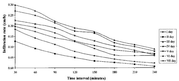
Fig.31 Infiltration rates of the clay loam soil at 60 mm/h rainfall intensity with 25 t/ha manure application rate.
