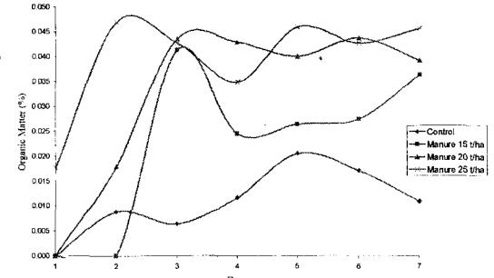
Fig. 48 Percentage of organic matter in the runoff water from elay loam soil at 30 mm/h rainfall intensity.
