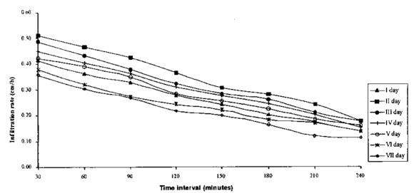
Fig. 5 Infiltration rates of sandy loam soil at 30 mm/h rainfall intensity with 20 t/ha manure application rate.
