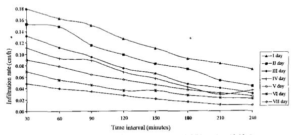
Fig.30 Infiltration rates of the clay loam soil at 60 mm/h rainfall intensity with 20 t/ha manure application rate.
