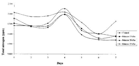
Fig.53 Total nitrogen content in the runoff water from sandy loam soil at 60 mm/h rainfall intensity
