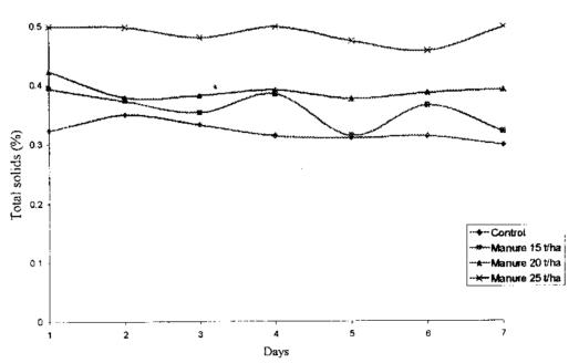
Fig.44 Percentage of total solids in the runoff water from clay loamsoil at 60 mm/h rainfall intensity.
