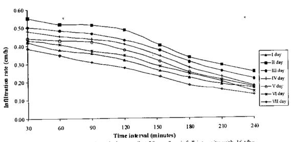
Fig. 4 Infiltration rates of sandy loam soil at 30 mm/h rainfall intensity with 15 t/ha manure application rate.
