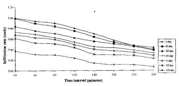
Fig. 10 Infiltration rates of sandy loam soil at 45 mm/h rainfall intensity with 20 t/ha manure application rate.
