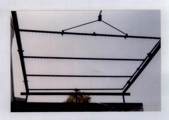
Plate II. Close view of the drop forming unit.
