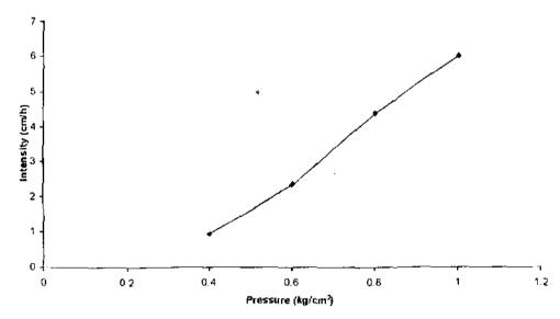
Fig. 2 Calibration curve for rainfall intensity of the simulator.
