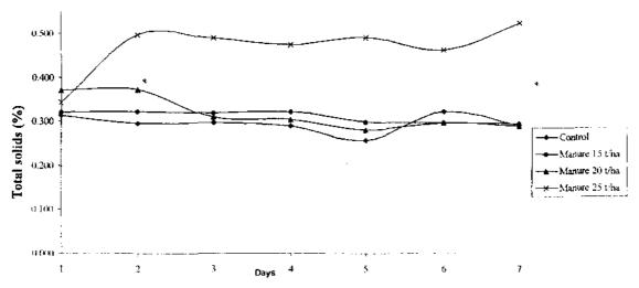
Fig.40 Percentage of total solids in the runoff water from sandy loam soil at 45 mm/h rainfall intensity.
