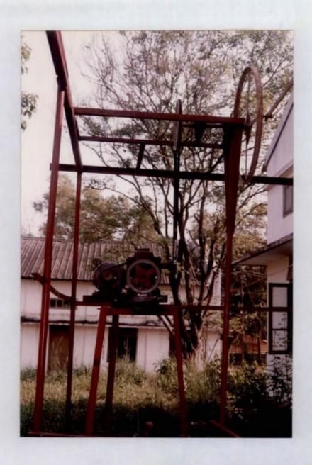
Plate III. Power transmission system of the rainfall simulator.
