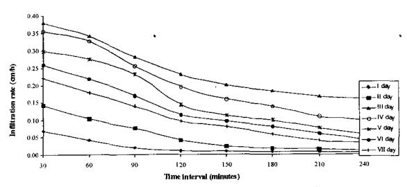
Fig. 20 Infiltration rates of clay loam soil at 30 mm/h rainfall intensity with 20 t/ha manure application rate
