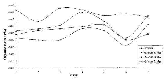
Fig. 49 Percentage organic matter content in the runoff water from clay loam soil at 45 mm/h rainfall intensity.
