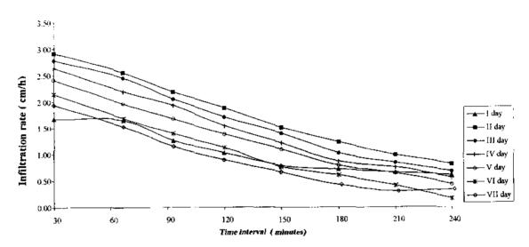
Fig. 13 Infiltration rates of sandy loam soil at 60mm/h rainfall intensity without manure.
