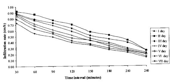
Fig. 3 Infiltration rates of sandy loam soil at 30mm/h rainfall intensity without manure.
