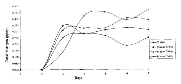
Fig.51 Total nitrogen content in the runoff water from sandy loam soil at 30 mm/h rainfall intensity.
