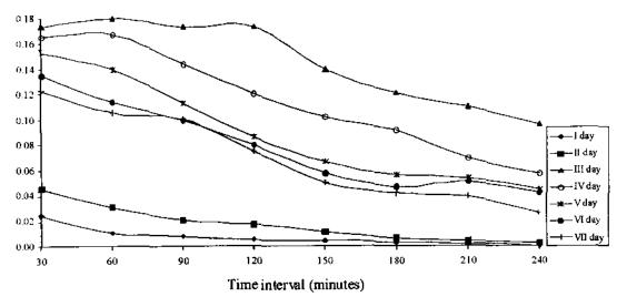
Fig. 19 Infiltration rates of clay loam soil at 30 mm/h rainfall intensity with 15 t/ha manure application rate
