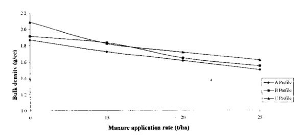
Fig.62 Bulk density values of clay loam soil at different profile levels under 60 mm/h rainfall intensity.
