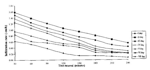
Fig. 15 Infiltration rates of sandy loam soil at 60 mm/h rainfall intensity with 20 t/ha manure application rate.
