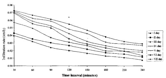
Fig. 28 Infiltration rates of the clay loam soil at 60 min/h rainfall intensity without manure.
