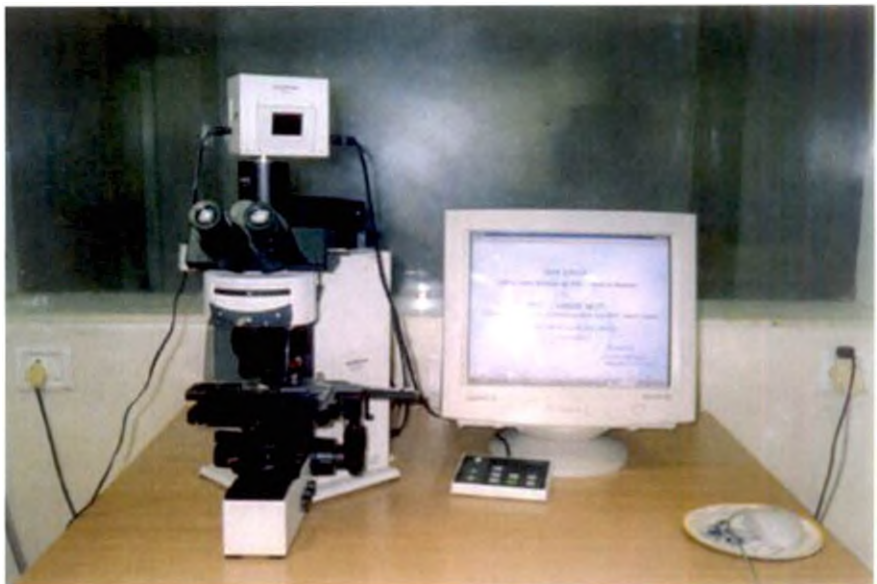
Fig. 5. Fluorescent microscope attached to the computer
