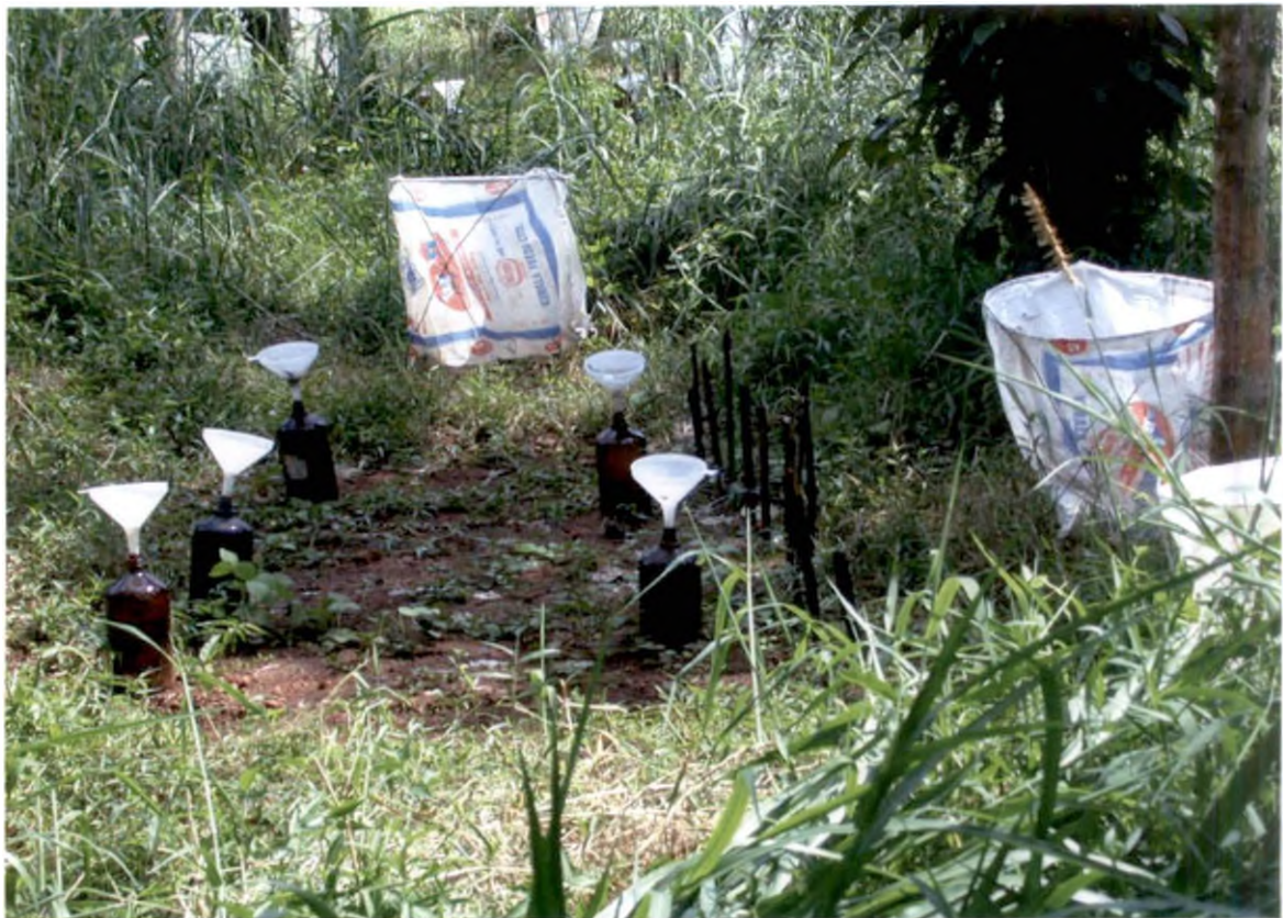
Plate 3 Litter trap along with the litter bags tied to pegs and rainwater measuring bottles
