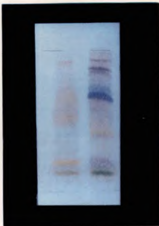
Plate 13: TLC plate of Limnophila repens and Bacopa monnieri Solvent system: EtOAc-MeOH-H 2 O
