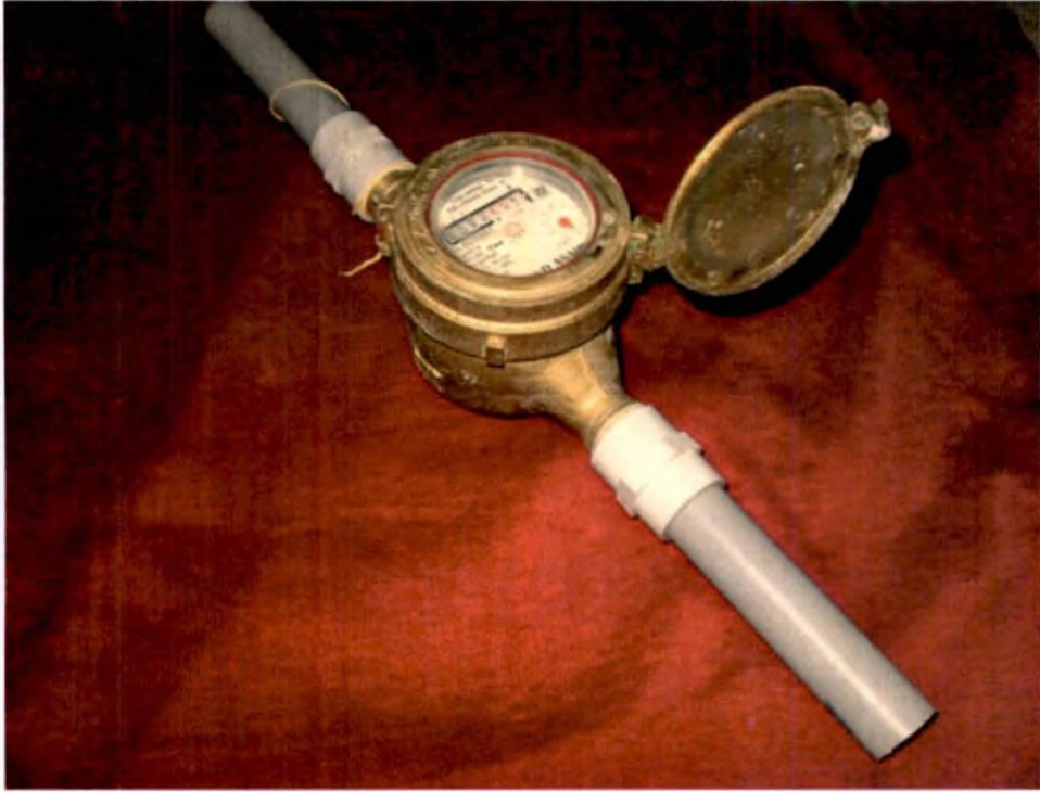
Plate 2. Water meter for irrigating with measured quantity of water
