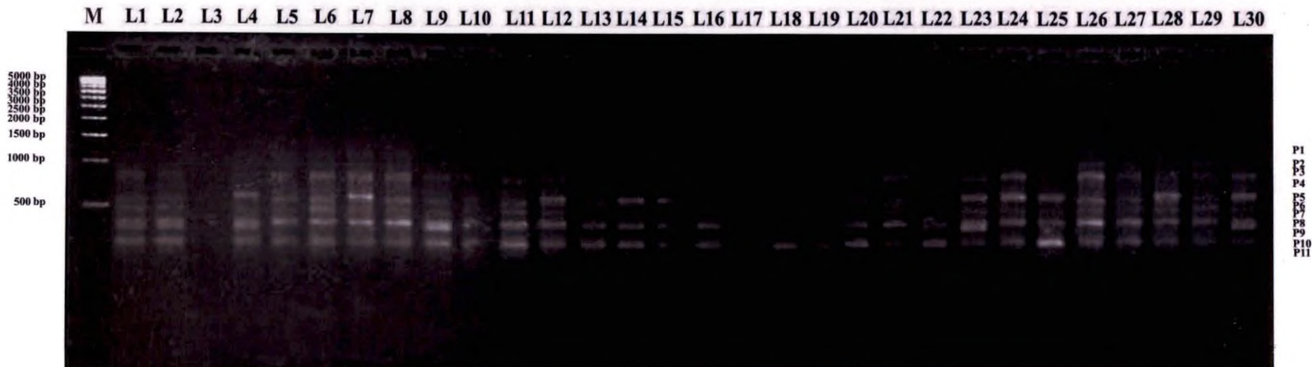
Plate 17. Amplification profile of the DNA of thirty rice accessions using the primer OPG-19
