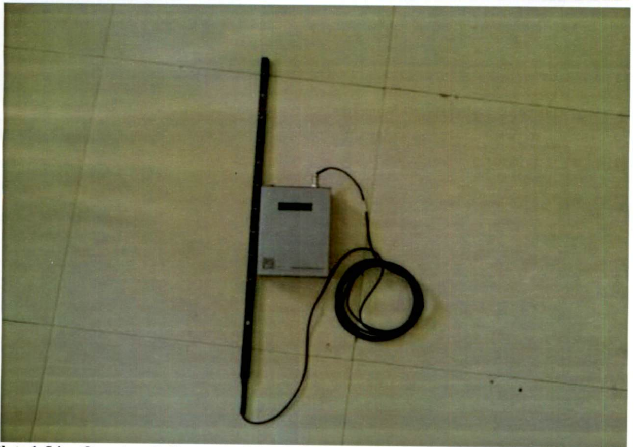
Plate 1. Line Quantum Indicator used for estimating understorey PAR in 7 year old bamboo ( Dendrocalamus strictus ) in Vellanikkara, Thrissur
