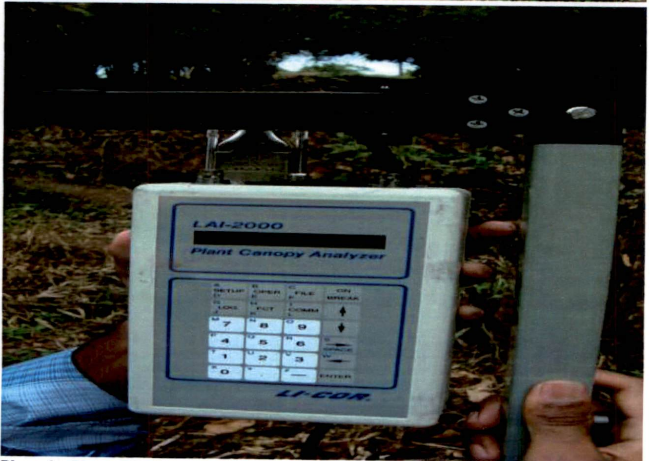
Plate 2. Plant Canopy Analyzer used for estimating LAI of 7 year old bamboo ( Dendrocalamus strictus ) in Vellanikkara, Thrissur
