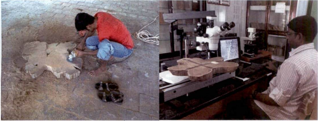
Plate 2. A. Polishing of wooden basal disc B. Measurement of ringwidth using tree ring station and stereo microscope
