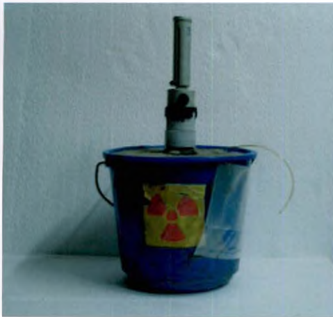
Plate 4. Device for soil injection of ^{32}\text{P} solution
