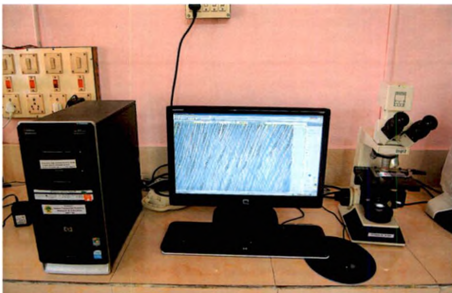
Plate 9. Image Analyser (Labomed Digi-2) used for anatomical quantification
