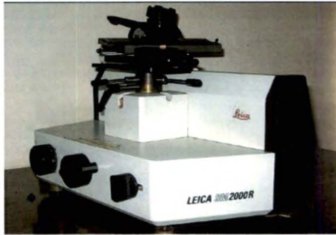
Plate 8. Sliding wood microtome (Leica SM 2000 R) used for wood sectioning
