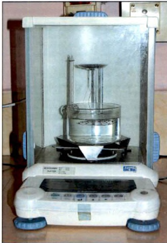
Plate 4. Specific gravity module attached to electronic balance (Schimadzu AU220)
