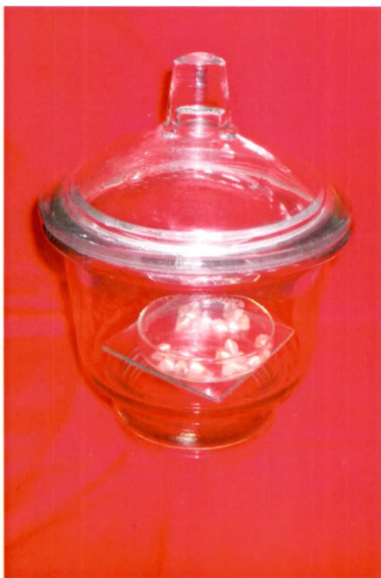
Plate 3. Desiccator with desiccation medium and synthetic seed
