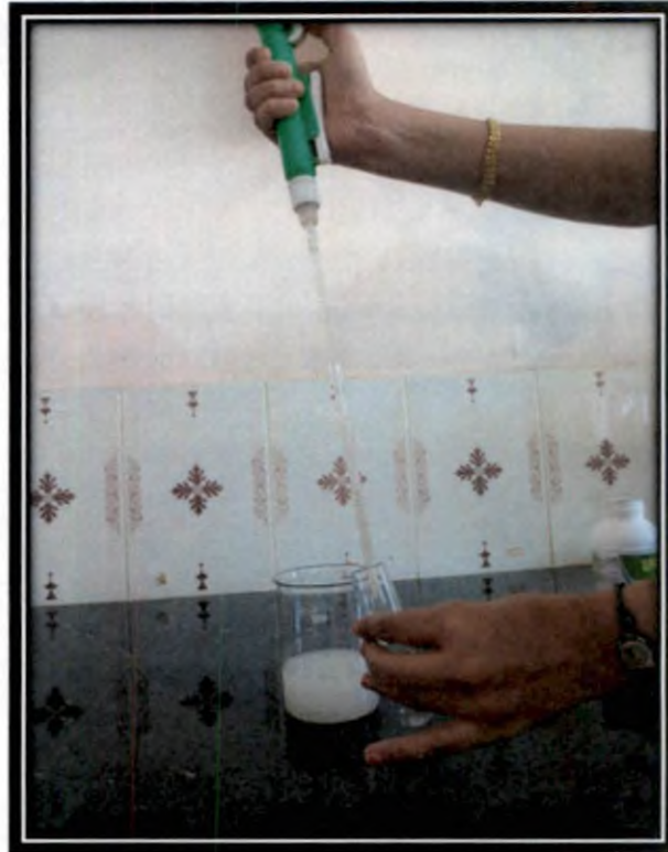
Plate 5. Preparation of field recommended concentration of insecticides using micropipette
