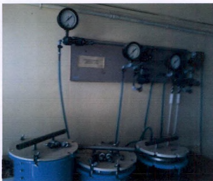
Plate 3.12 Pressure plate and pressure membrane apparatus
