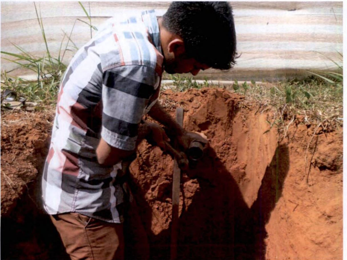
Plate 10. Bulk density estimation using steel cylinder
