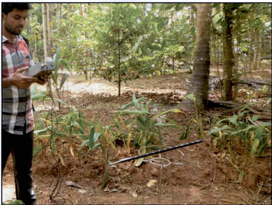
Plate 4. Line quantum sensor established in the homegarden
