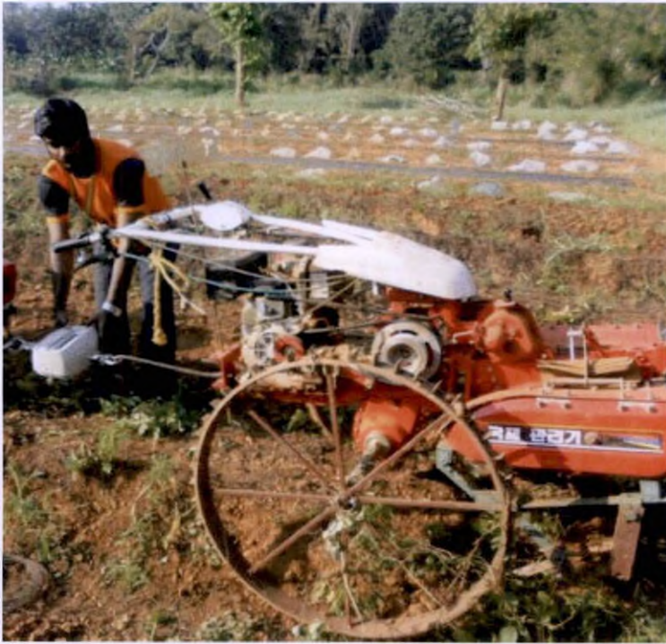
Plate 3.8 Testing of modified coleus harvester
