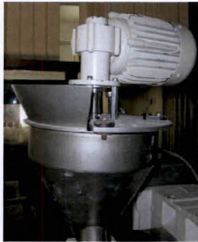
Plate 3.12 Feed hopper of a brabender extruder
