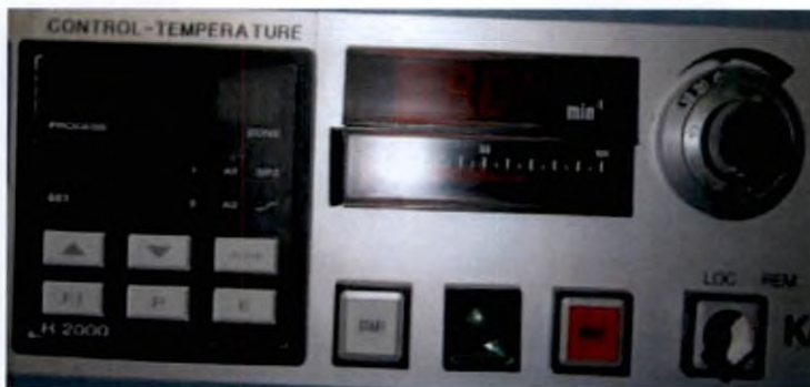
Plate 3.13 Digital torquemeter of a brabender extruder
