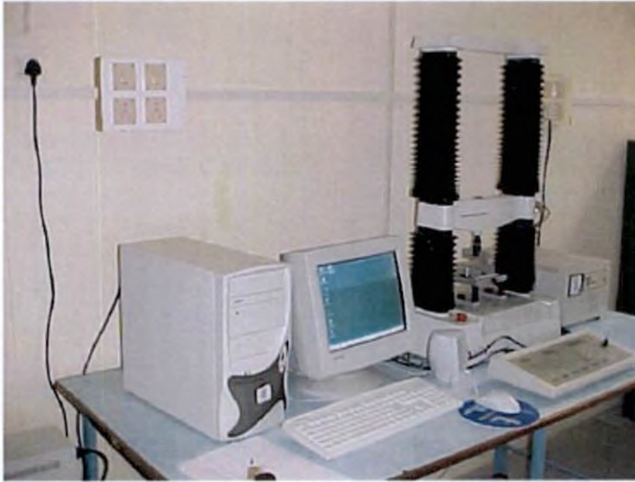
Plate 3.9 Experimental set up of TA.XT plus texture analyser
