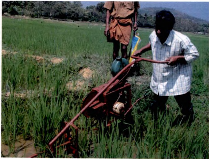
Plate 6. The self propelled cono weeder – Model 1
