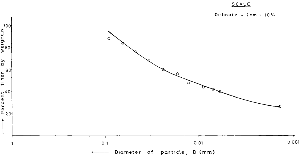
Fig-11 GRAIN SIZE DISTRIBUTION CURVE (Hydrometer Analysis)
