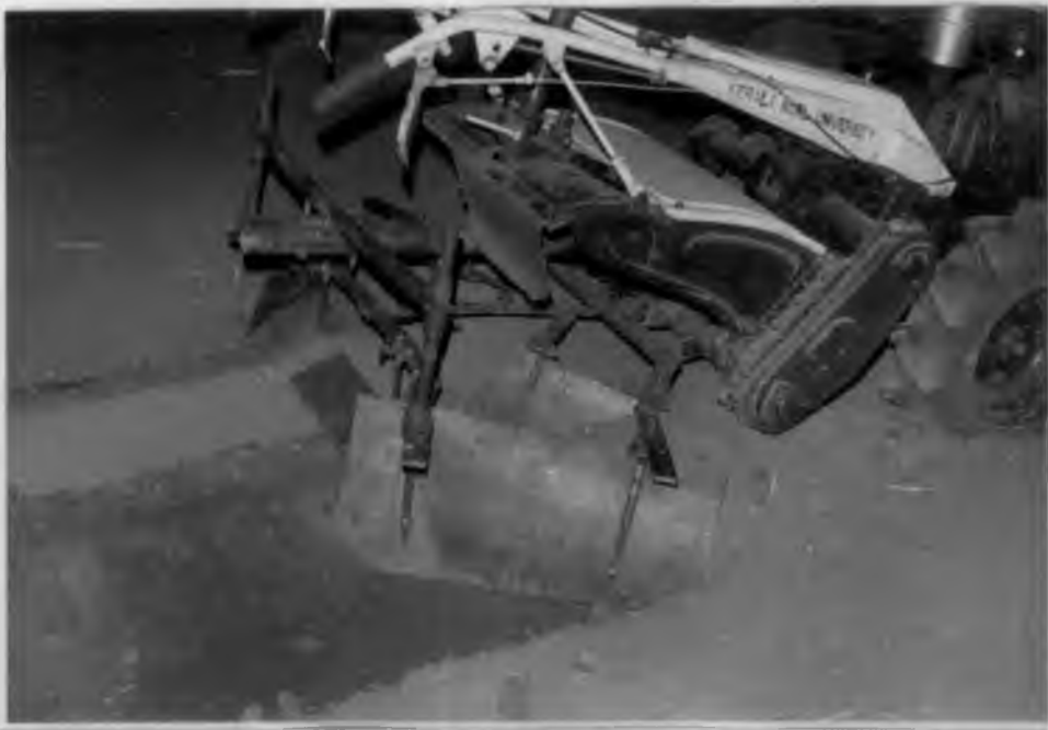
Plate IV Power tiller operated bed former in operation (side view)
