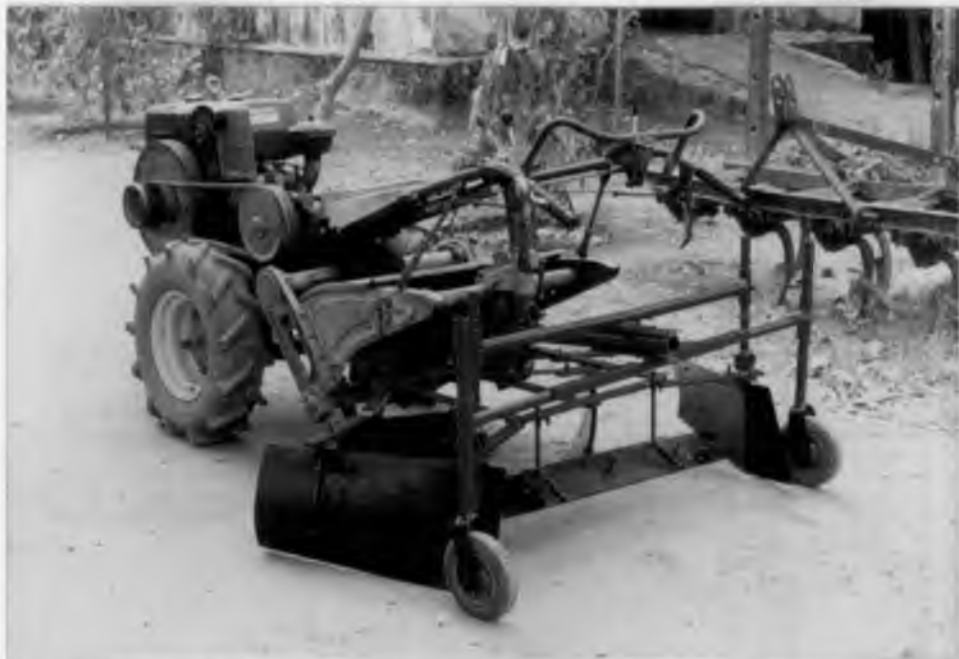
Plate VI Power tiller operated bed former attached with Kubota power tiller
