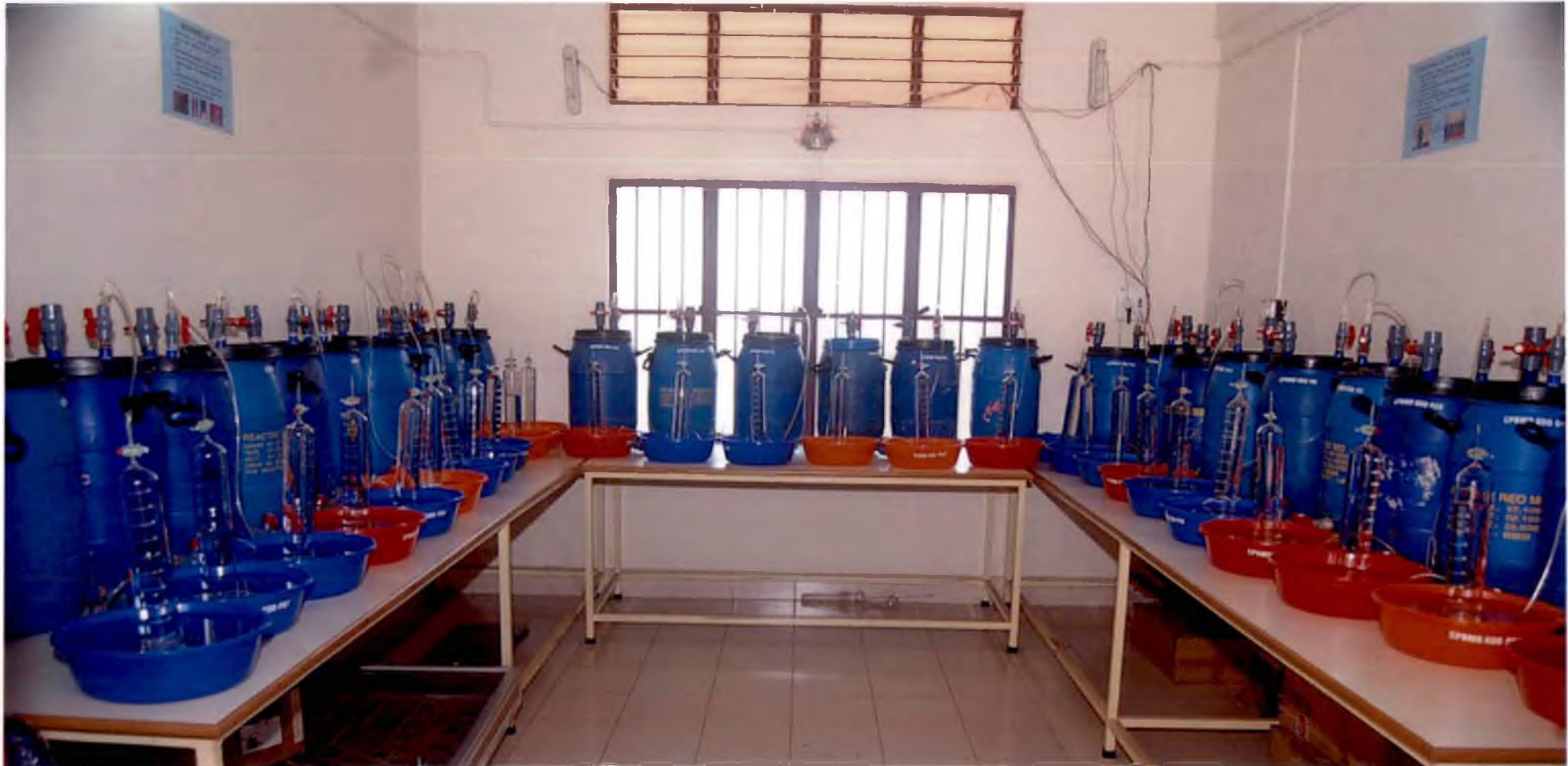
Plate 14. The biogas experimental setup developed for the study in Environmental Biotechnology Laboratory
