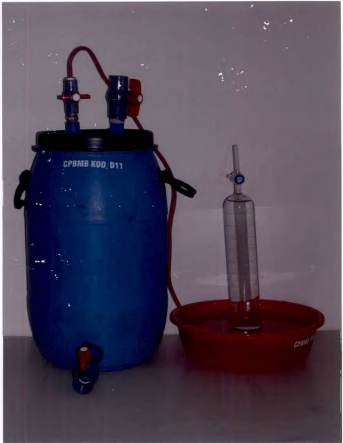
Plate 2. Experimental biogas unit
