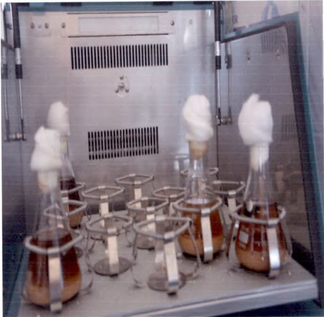
Plate 5 Incubation of powdered plant samples in shaking incubator for hydro-alcoholic extraction
