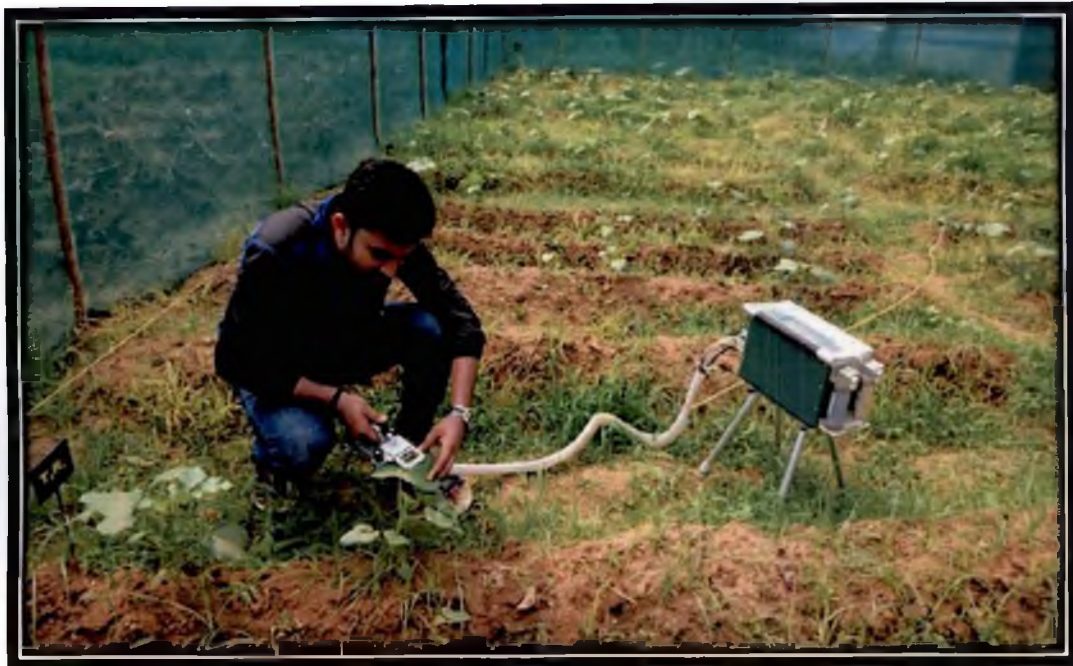
Plate 7. Measurement of gas exchange parameters by portable photosynthesis system
