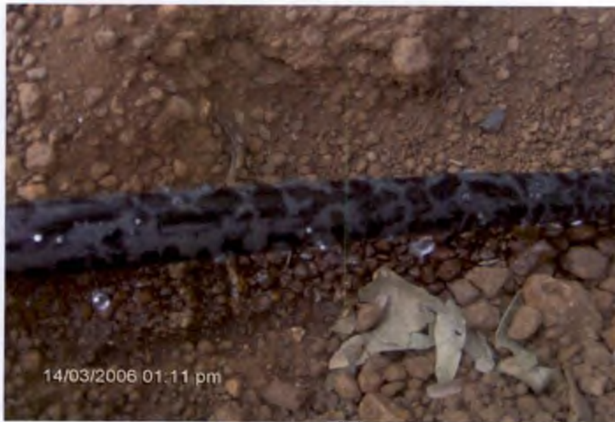
Plate 3.11 Porous Pipe Discharge Pattern
