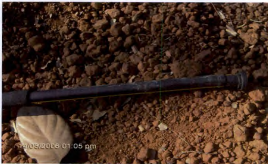
Plate 3.5. Flushing Device for Laterals
