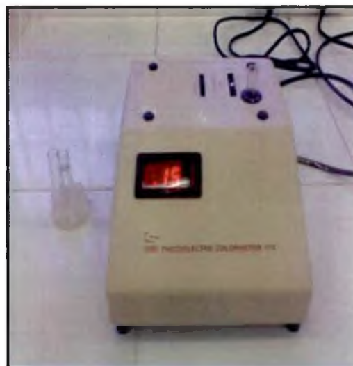
Plate 10 Photoelectric colorimeter used for determination of Phosphate.
