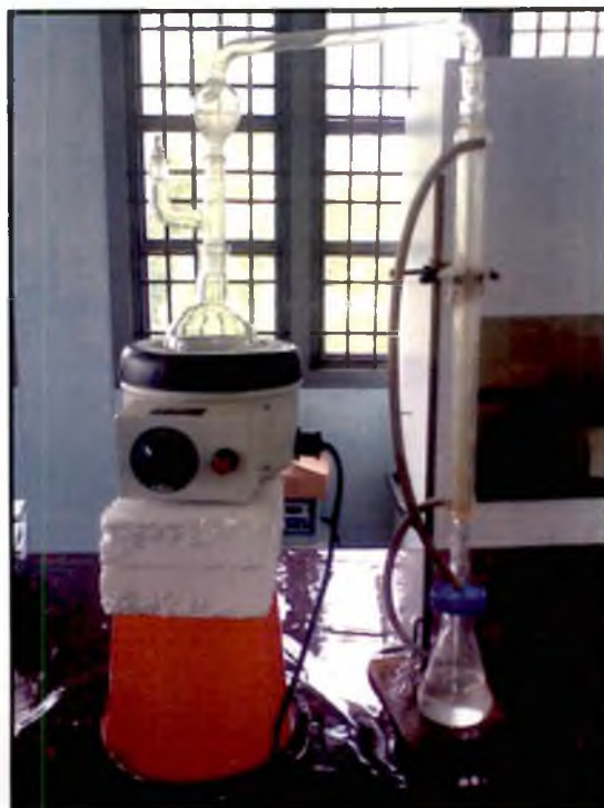
Plate 8 Experimental set up for distillation in determination of TKN.
