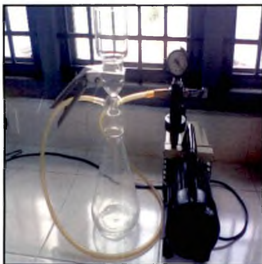
Plate 9 Filtration unit for determination of TSS.
