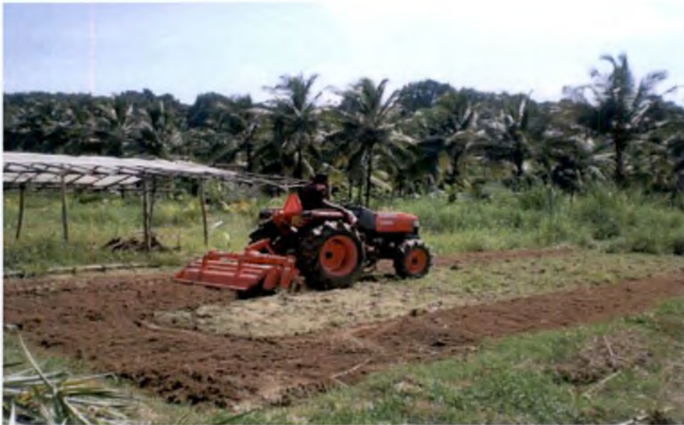
Plate 4. Land preparation by rotavator
