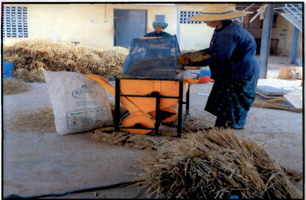
Plate 6. Threshing and winnowing of harvested produce with mechanical thresher cum winnower
