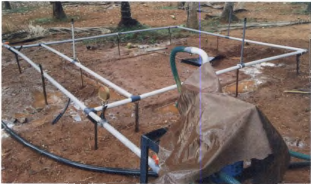
Plate 1. Installation of rainfall simulator on micro plot
