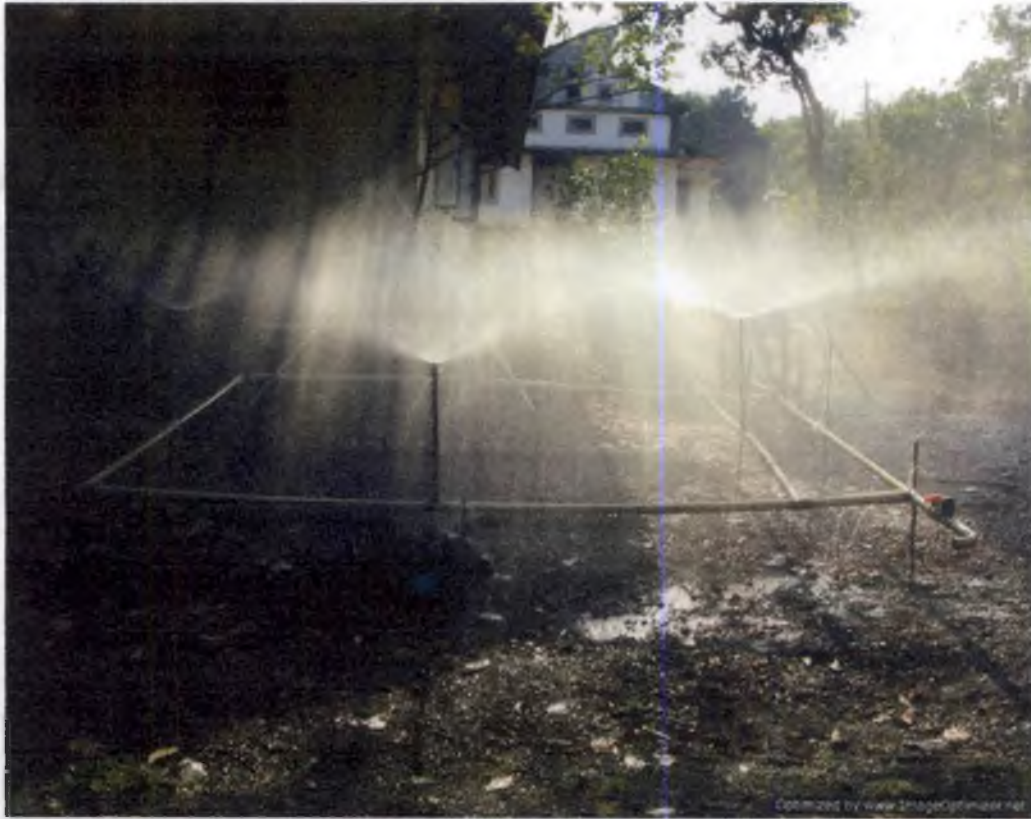
Plate 8. Rainfall simulator in operation on erosion plot
