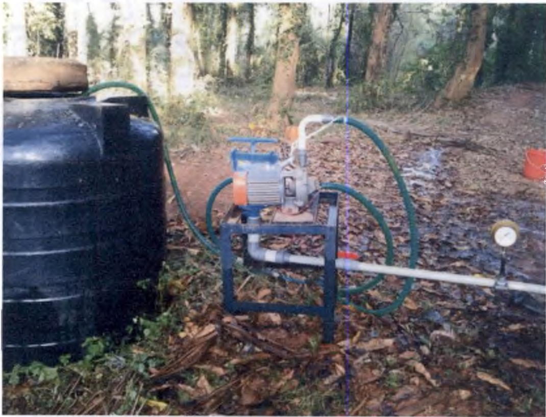
Plate 4. Water supply to the rainfall simulator
