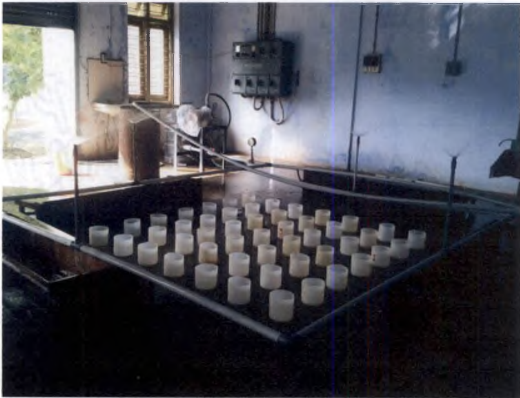
Plate 5. Rainfall simulator testing
