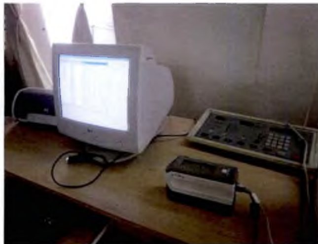
Plate 10. Spectrophotometer assembly for colour measurement
