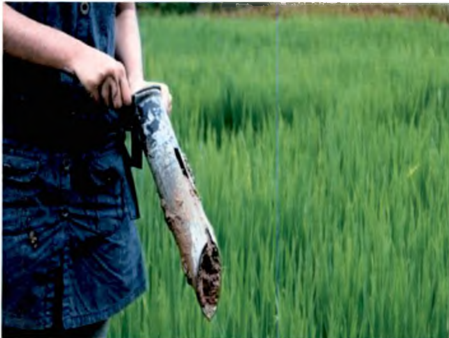
Plate 2. Soil samples collected using core sampler at a depth of 0 to 15cm
