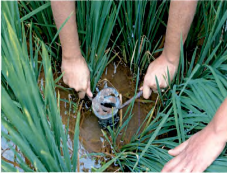
Plate 2. Soil samples collected using core sampler at a depth of 0 to 15cm
