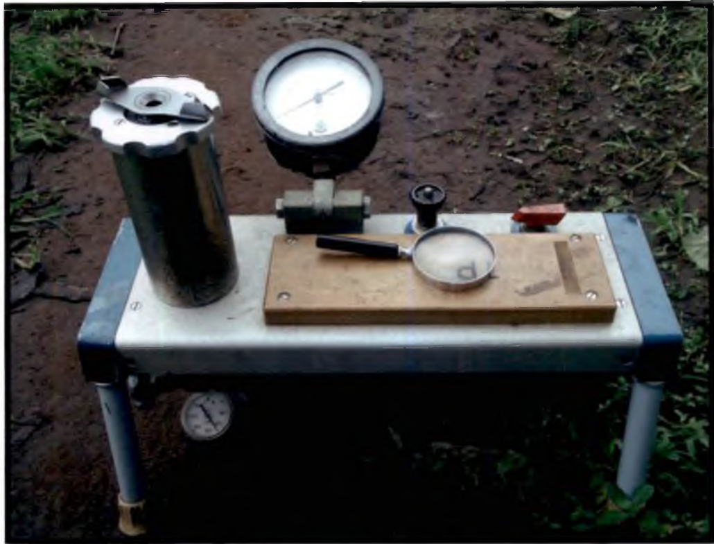
Plate. 3. Pressure bomb apparatus for measuring water potential
