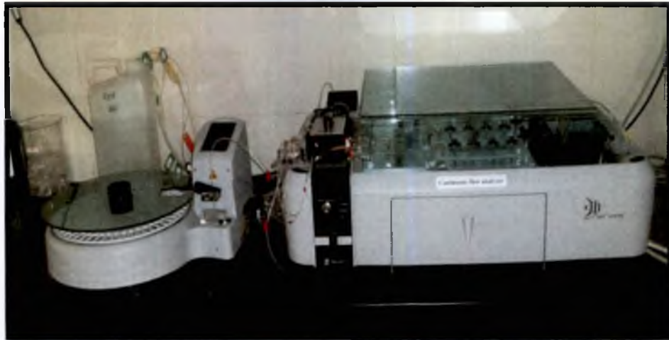
Plate 9. Continuous flow analyser (SKALAR) for estimation of N and P
