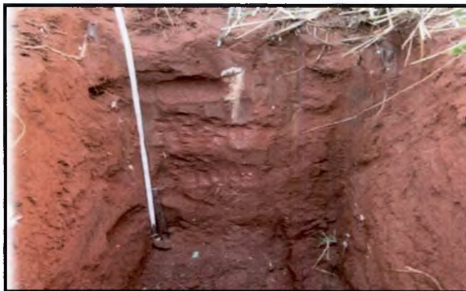
Plate 4. Soil profile for collecting samples for organic carbon and nutrient analysis
