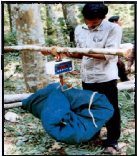
Plate 2. Weighing of different biomass components in the field using digital spring balance
