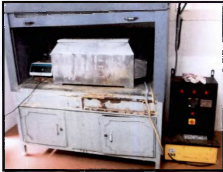
Plate 7. Digestion chamber for soil and plant sample digestion
