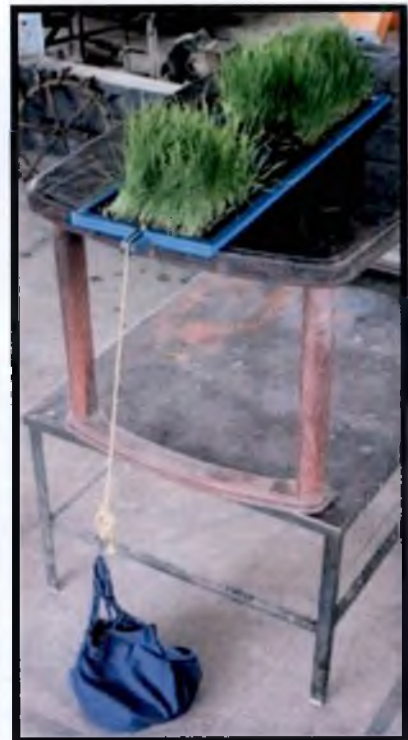
Plate 2. Instrument used for finding out mat strength
