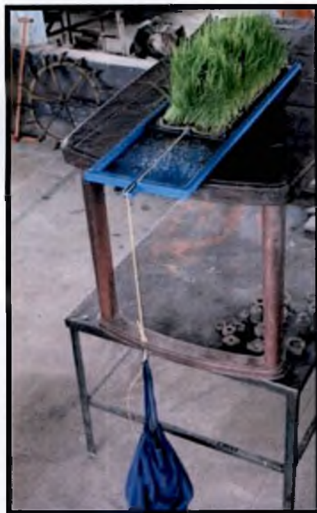
Plate 2. Instrument used for finding out mat strength
