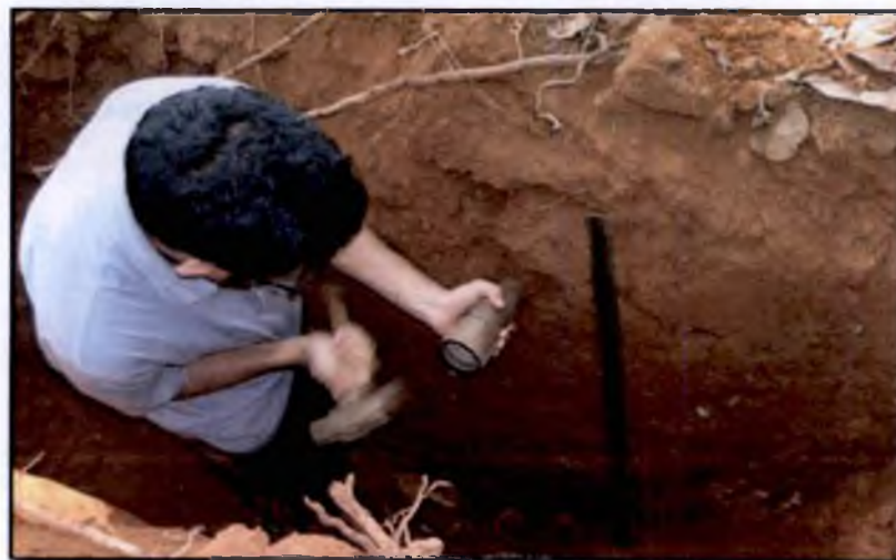
Plate 9. Taking a soil core for bulk density measurement
