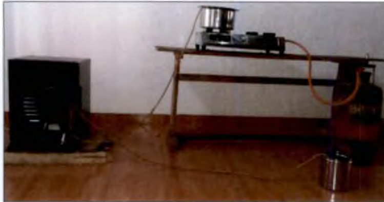
Plate 3.7 Setup for the performance of VARS using hot water generated in a steel vessel
