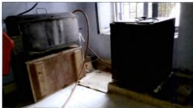
Plate 3.6 Setup for the performance of VARS using hot water from blancher
