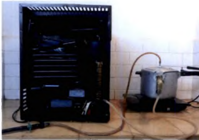
Figure 3.5 Set for the performance of VARS using steam (Hot water supplied by solar flat plate collector)
