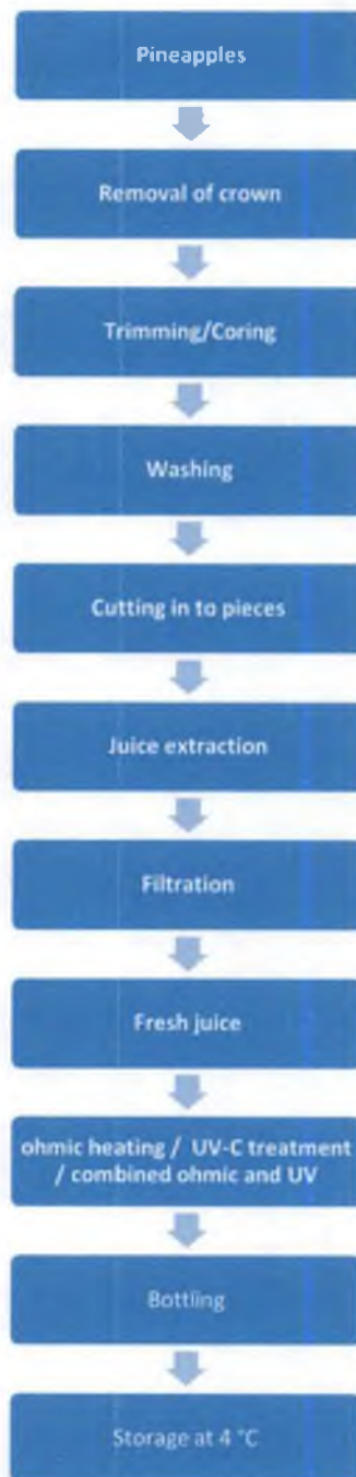
Figure 3.2 Process flow chart for production of treated pineapple juice
