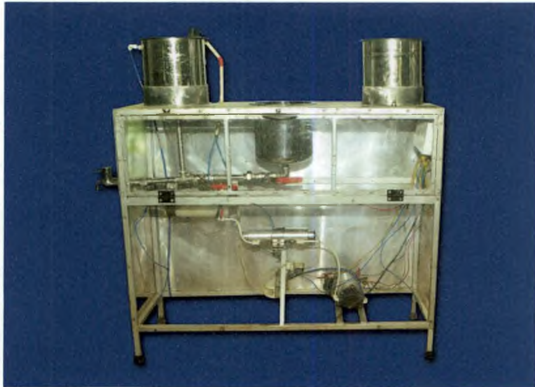
Plate 3.1 Developed combined Ohmic heating and UV treatment apparatus
