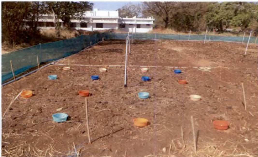
Plate 4. Estimation of distribution uniformity of sprinkler by catch can method
