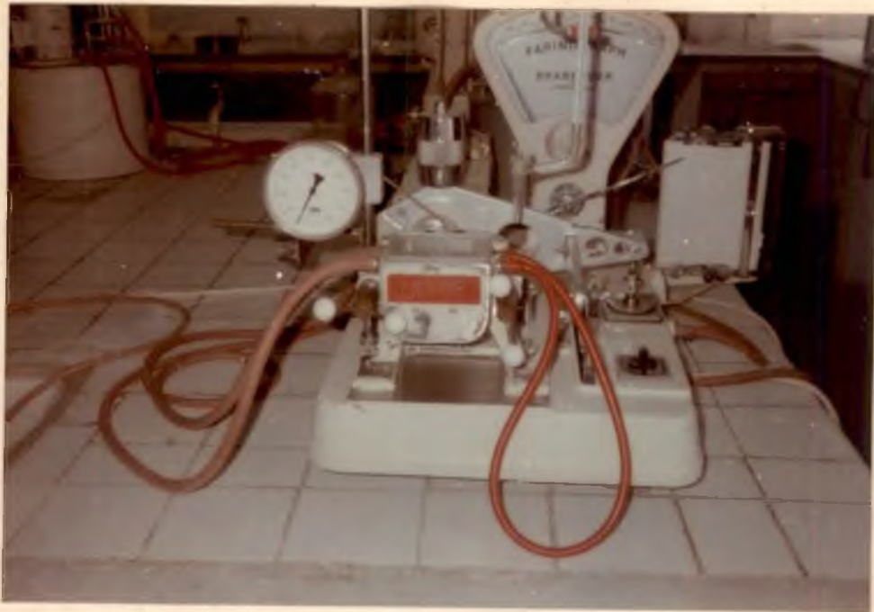
FIG.8 - EQUIPMENT USED FOR TESTING WATER ABSORPTION
