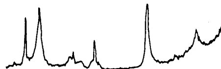
Fig. 11. X-ray diffraction pattern of the <2\ \mu\text{m} fraction of surface samples of major wetlands of Kerala - KATTAMPALLY
