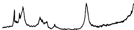
Fig. 10. X-ray diffraction pattern of the <2\ \mu\text{m} fraction of surface samples of major wetlands of Kerala - PATTAMBI
