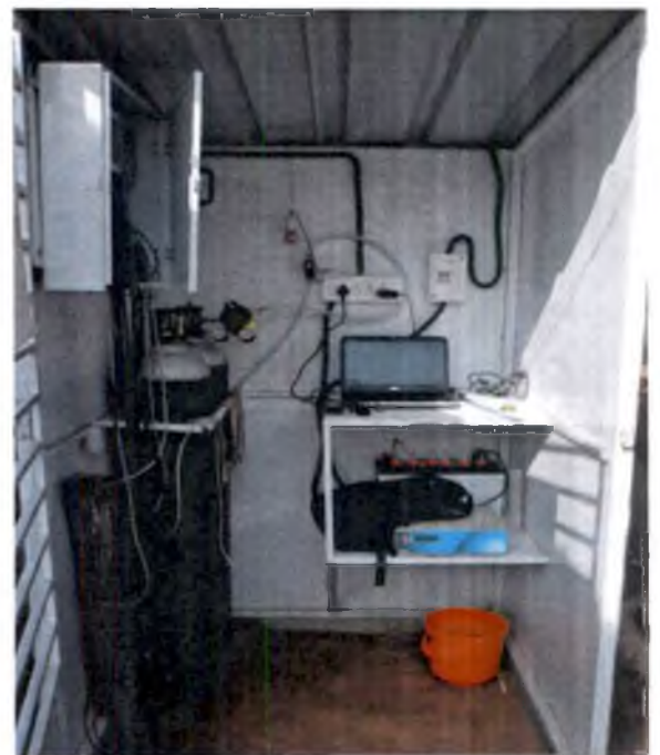
Plate 1. Open Top Chamber system for CO 2 enrichment
