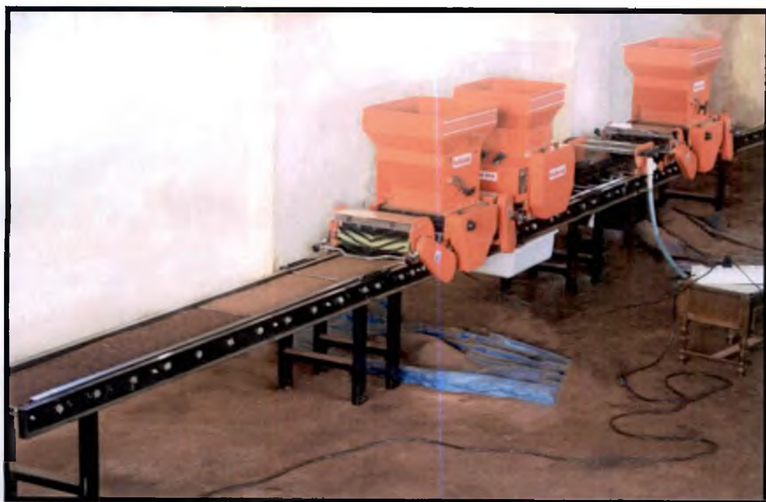
Plate 1. Filling of trays using Automatic Rice Mat Nursery Sowing Machine
