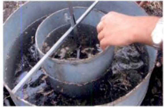
Plate 7. Measurement of infiltration rate
