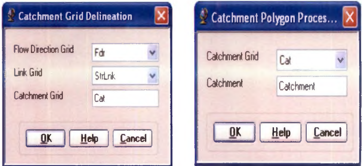
Fig 3.16. Snapshot of creation of catchment grid delineation, catchment polygon processing in HEC-GEOHMS
