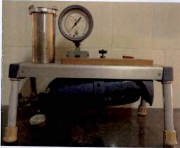
Plate 5. Measurement of plant water status using pressure bomb apparatus.
