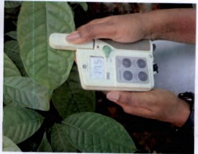
Plate 6. Measurement of chlorophyll content using SPAD meter.
