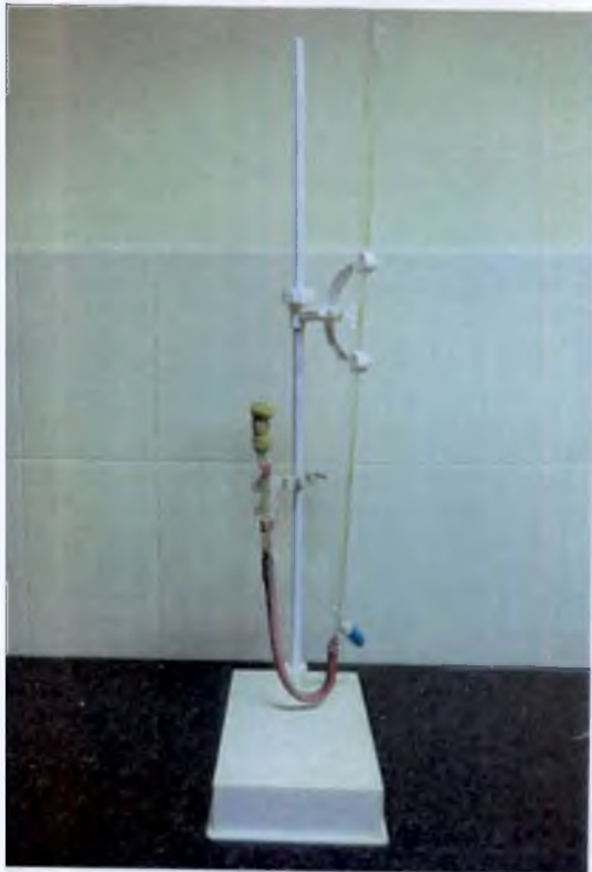
Plate 7. Piche's evaporimeter used for measuring evapotranspiration.
