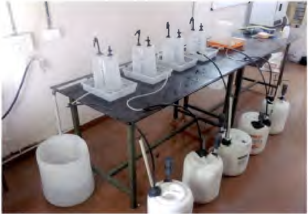
Figure 6. Arrangements of batch digesters for study
