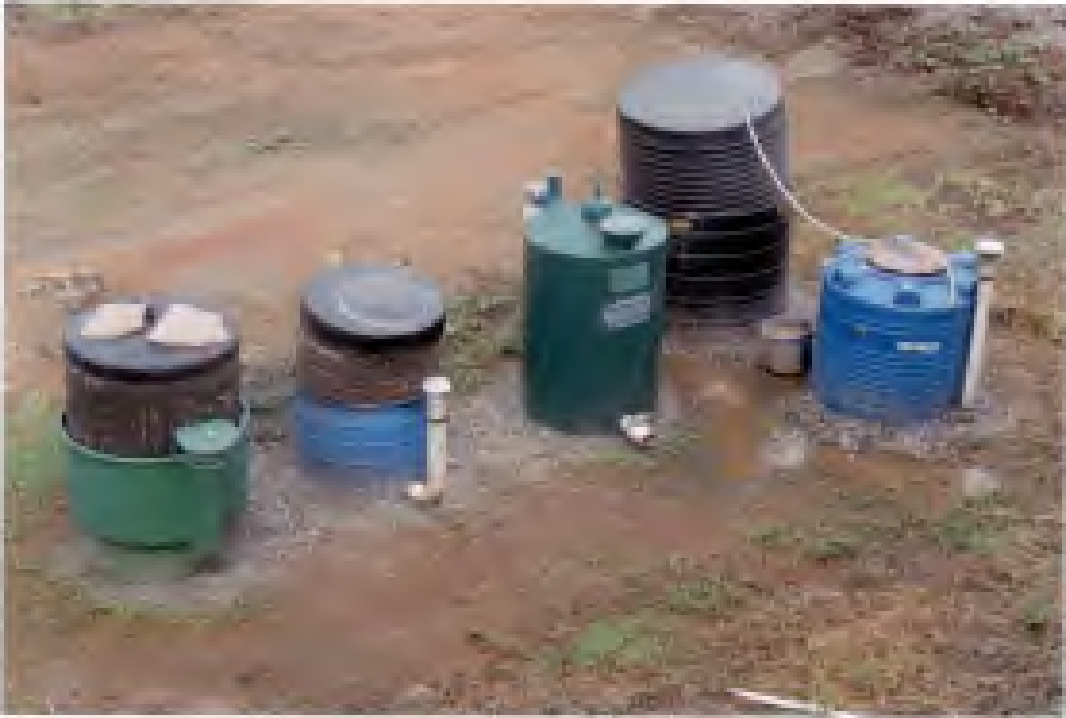
Figure 16. Layout of Portable Biogas Plants
