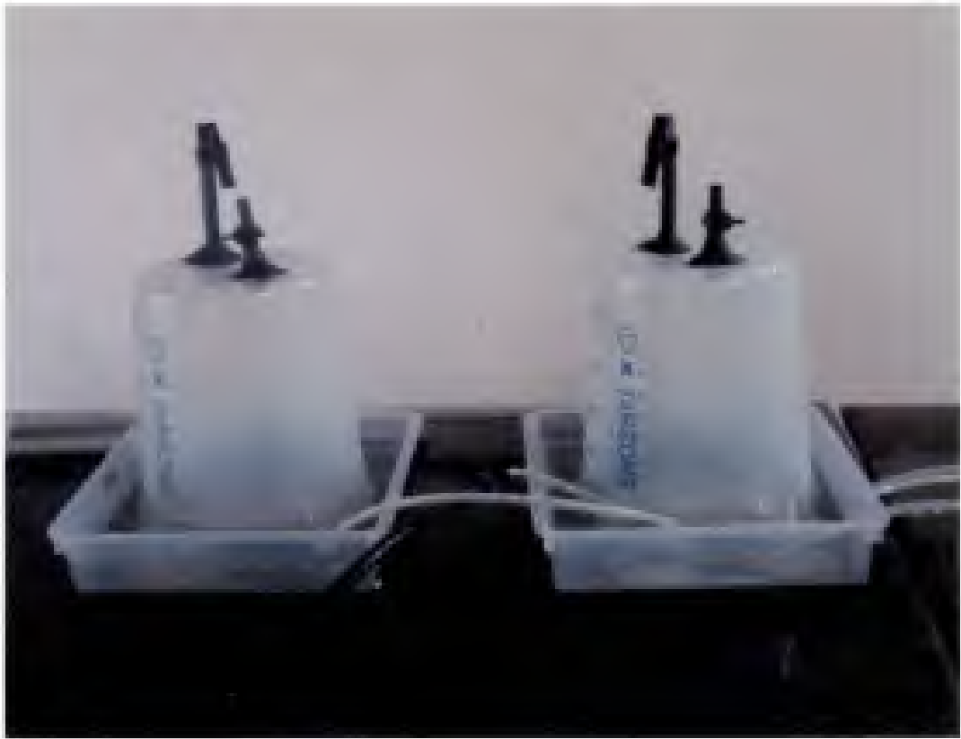
Figure 3. Water displacement meter
