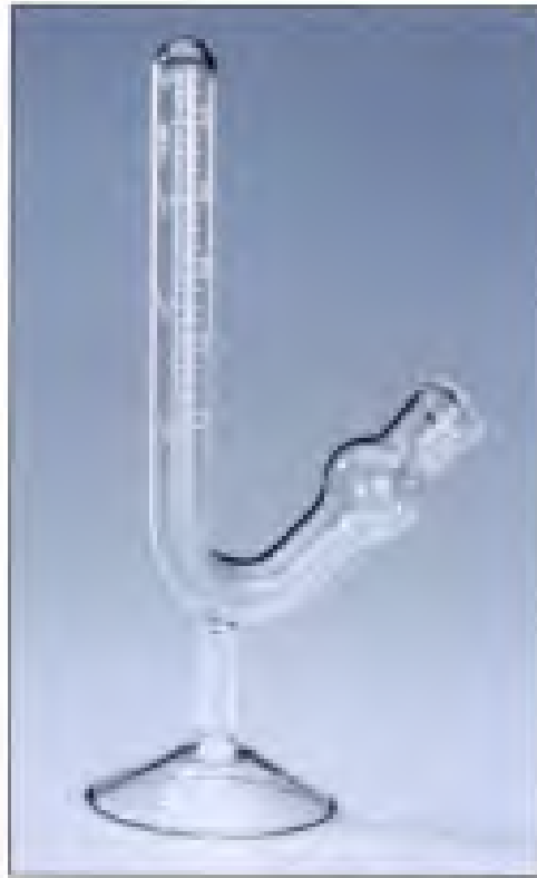
Figure 9. Saccharometer for measuring the methane content of biogas
